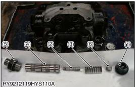
11. Install the counterbalance unit. Install the plunger (counterbalance) and metal washer (spring) in order.
