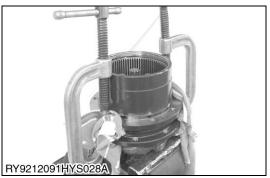
13. Use a vice or hydraulic press to press the flange holder and gear case together.
