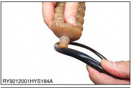
9. Apply grease to the O-ring of the seal and install the seal.
