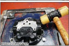
8. Tap the body (counterbalance) with a plastic hammer to raise it. Insert a slotted screwdriver into the gap and tap the body (counterbalance) from the opposite side with the hammer to remove it.
