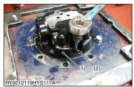
7. Install the piston Assy into the plate (retainer) and then install it into the cylinder block.
