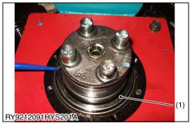
12. Apply a little gear oil to the sliding surface of the floating seal. (4 places, every 90 °)
