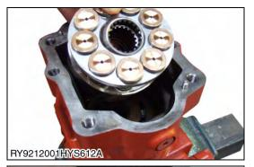
11. Remove the cylinder block ASSY.
