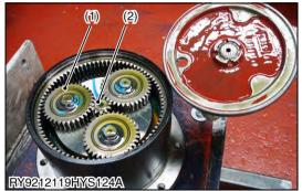
17. Install the holder, sub-assembly and sun gear.
