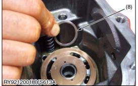
12. Remove the thrust washer (8).
