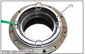
7. Apply a little gear oil to the sliding surface of the seal. (4 places, every 90°)
