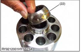
10. Install the retainer holder (22) onto the cylinder block.
