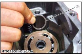
5. Attach the valve ASSY to the case.
