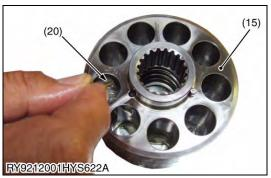
9. Insert the three pins (20) into the cylinder block (15).
