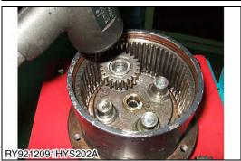
15. Gently tap the planetary gear into place with a plastic hammer.
